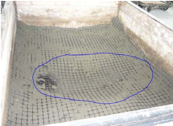
Figure 4.b. Failure surface on the reinforced scale model
