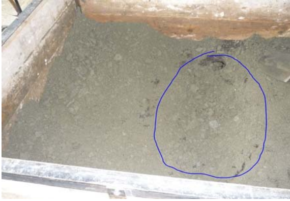
Figure 4.a. Failure surface on the unreinforced scale model
