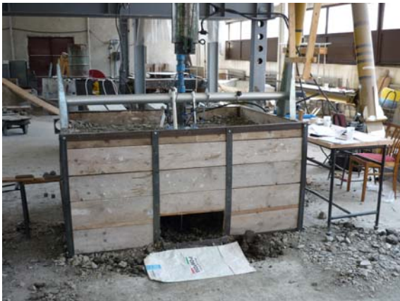
Figure 3. Lucas plate testing on the laboratory model
