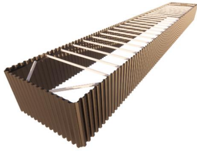
Figure 1 BIM model of the sheet pile wall
