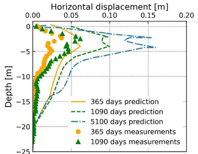
Figure 4. Horizontal displacements of the embankment toe
