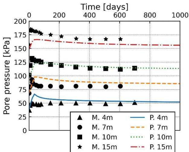
Figure 3. Dissipation of pore pressure at four depths under the embankment centre. M. is measurements, P. is prediction
