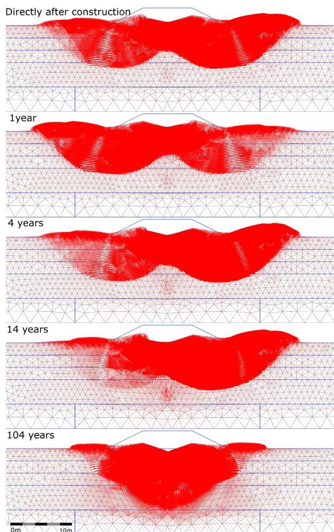
Figure 6. Total displacements vectors under the embankment at failure for the different time steps. Same scale for all time steps, scale in meter
