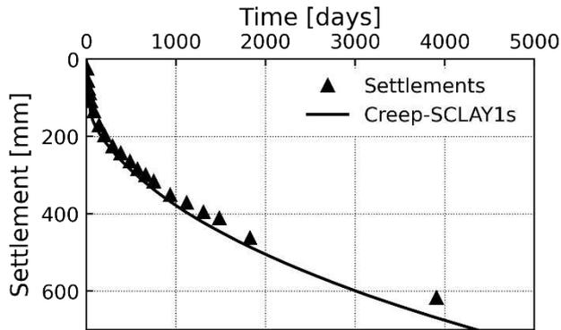
Figure 2. Settlement of under the centreline of Haarajoki embankment. Simulation and data from Hernvall et al., (2021)
