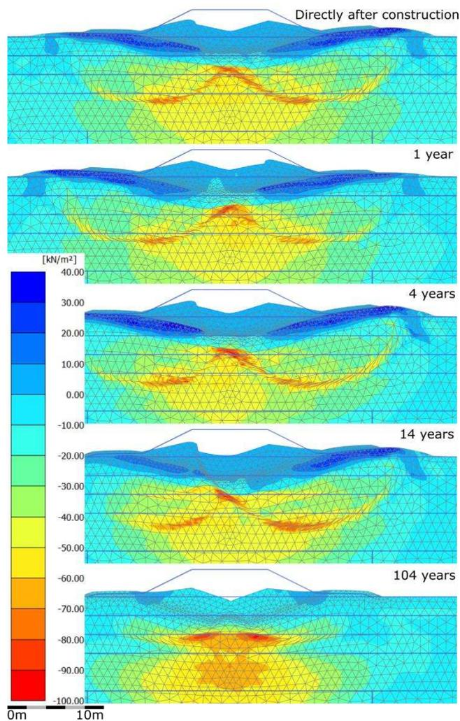
Figure 8. Excess pore pressure at failure for the different time steps
