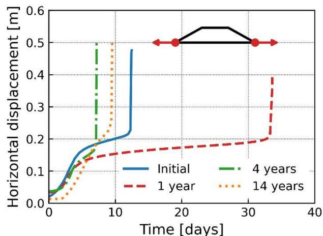
Figure 7. Horizontal displacement of the embankments toe at the different time steps
