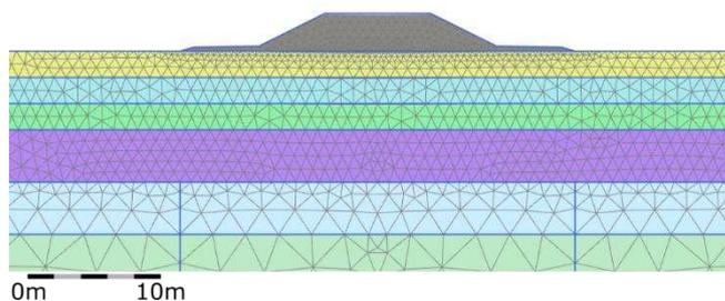
Figure 1. The mesh used for the calculation
