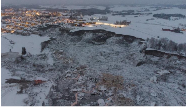
Figure 3. Retrogressive landslide in the sensitive clays of Gjerdrum in Eastern Norway on December 30, 2020 (Photo: Anders Martinsen)
