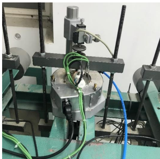
Figure 1. Consolidation cell modified for controlled-temperature testing.
