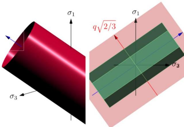
Figure 2. Von Mises and Tresca yield/failure surfaces visualised on the 'Animating Soil Models' project's page: [\[Link\]](#)
