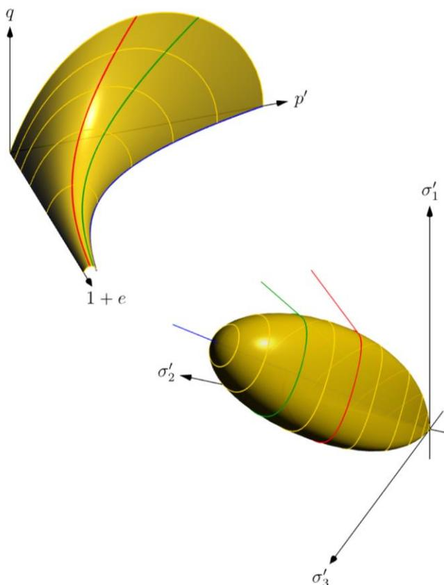
Figure 7. Asymptotic state boundary surface (ASBS) of clay hypoplasticity in  $p'$ - $q$ - $e$  space (left) and principal stress space (right) [\[Link\]](#)
