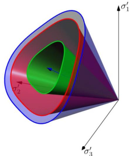
Figure 8. The dilatancy, critical state, bounding surfaces of SANISAND plasticity are visualised. More interactive visualisations and a video can be online: [\[Link\]](#)
