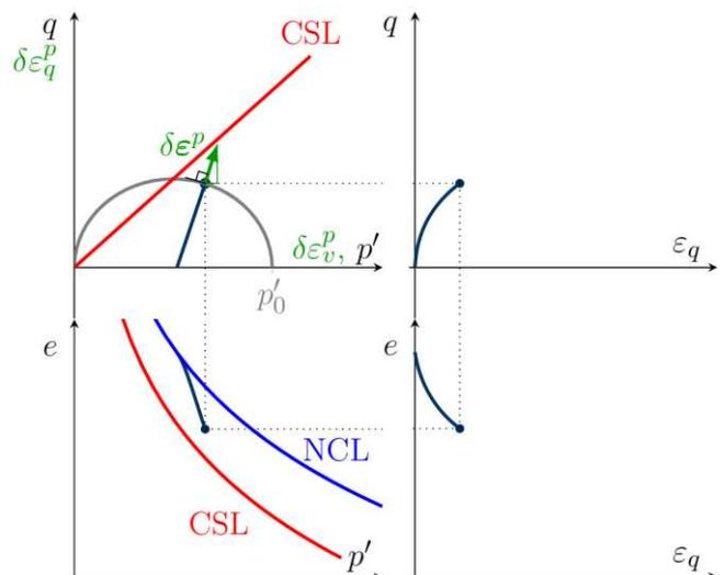
Figure 5. Example Modified Cam Clay Model of a normally consolidated drained triaxial compression test: [\[Link\]](#)
