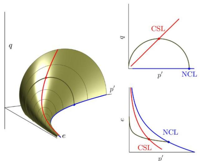
Figure 6. State boundary surface (SBS) of the MCC model. The linked interactive graphic allows to vary the parameters that control the shape of the SBS. [\[Link\]](#)
