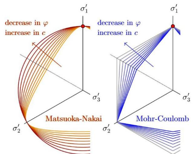
Figure 3. How do the parameters  $c$  and  $\phi$  influence the shapes of the failure surfaces Matsuoka-Nakai and Mohr-Coulomb? [\[Link\]](#)
