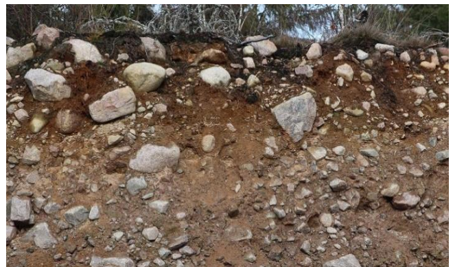
Figure 2. An excavation into a moraine layer, showing the boulders and the surrounding soil.
