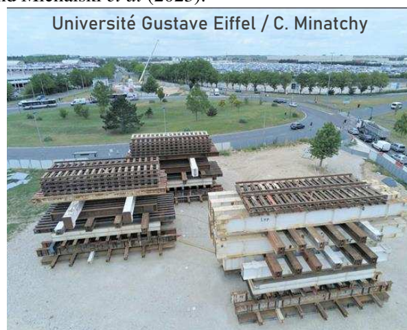
Figure 1. View of the experimental site and of the three steel frames used to load the piles
