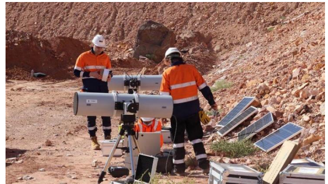
Figure 3. Two muon detector telescopes mid-installation (note not their final placements), with the background muon counter as the small black box at its base.
