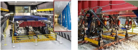
Figure 1. General view of the CEDEX Track Box and the hydraulic actuators.
