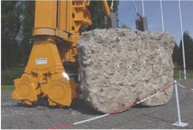
Figure 1. CSM equipment with rotation around horizontal axes and view of a CSM panel.
