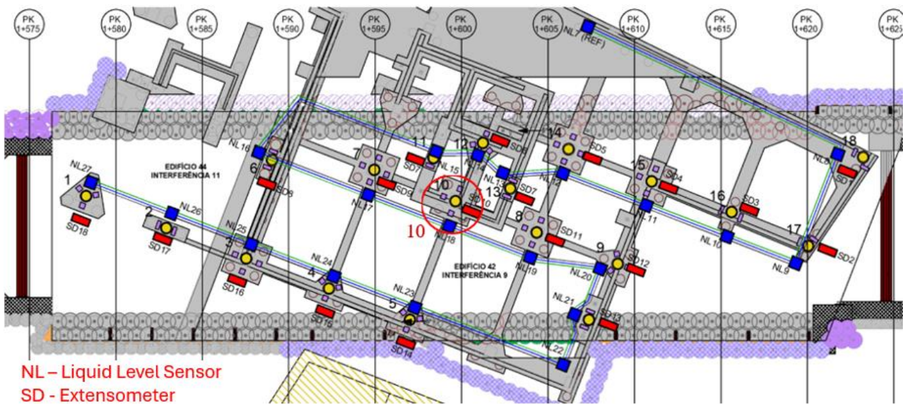
Figure 6. Lisbon Metro line new circular line: Underpinning building - Monitoring devices.
