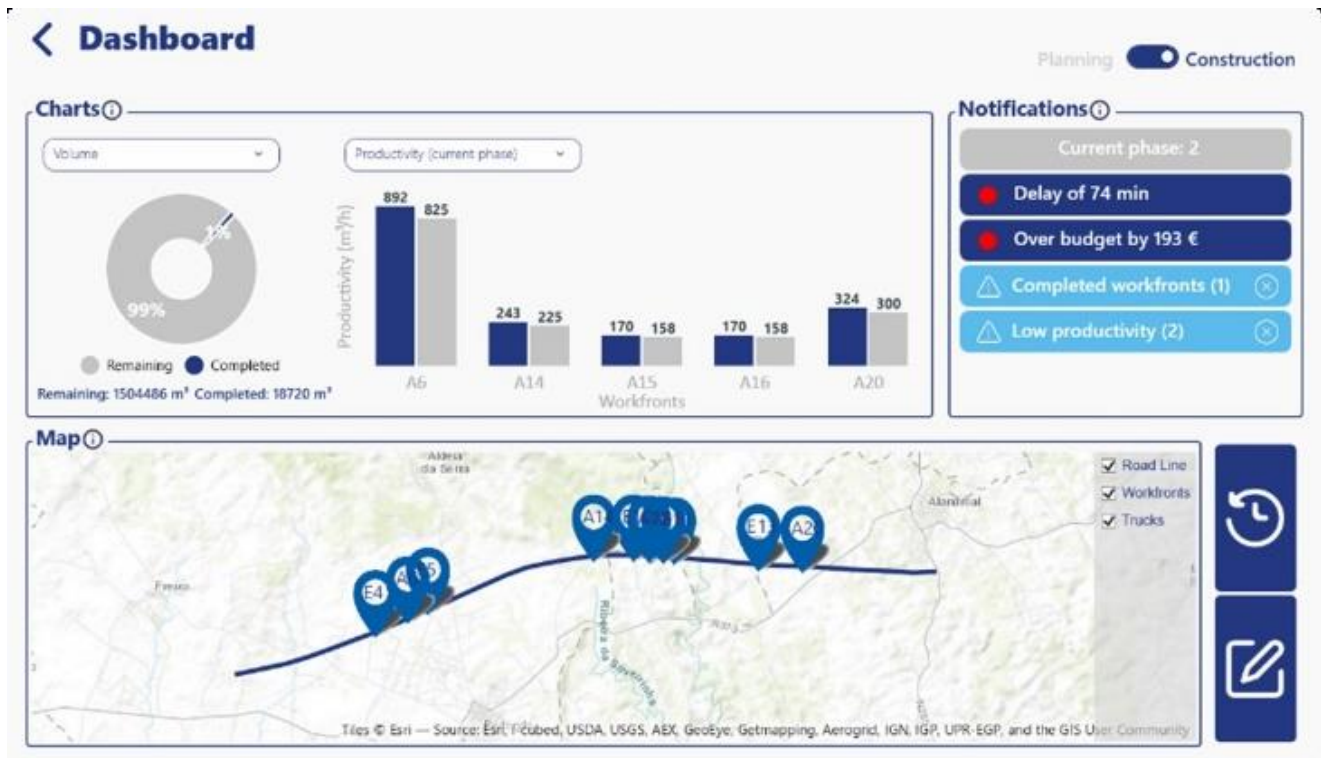
Figure 3. Monitoring and control dashboard for the conducted construction simulation.
