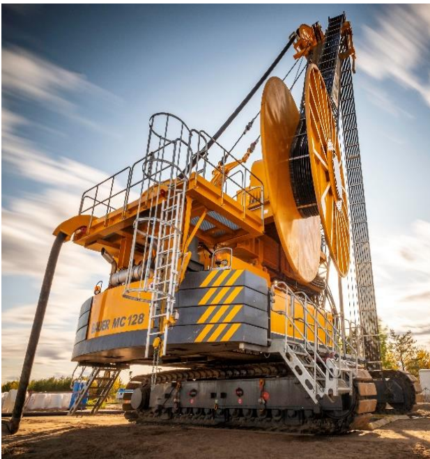
Figure 7. Cutter system for great depth up to 250 m.
