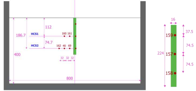
Figure 1. Experimental setup showing the model wall and the positions of total stress sensors in the sand and on the wall shaft.
