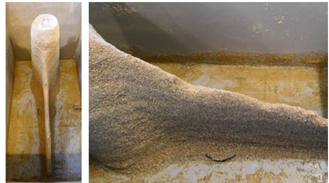
Figure 6. Exposed cement/sand plume of the model pile from cement suspension in sand2: v_f = 290 m/day (Fierenkothen et al., 2020).
