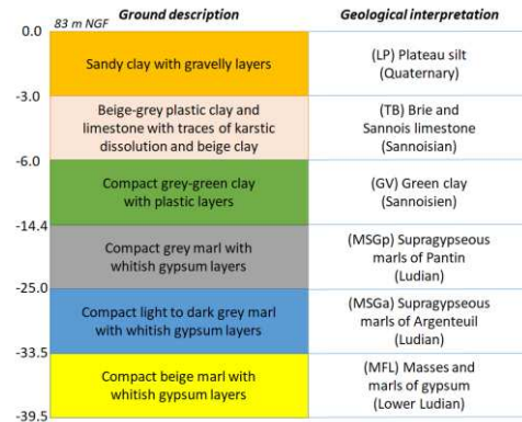
Figure 1. Geological profile (scale not observed). 83 NGF correspond to the surface of the work site.
