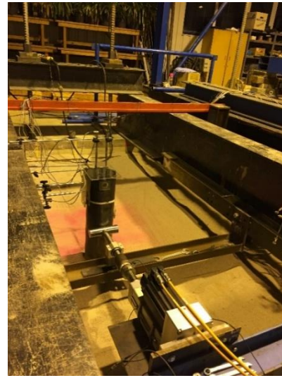
Figure 4. Lateral cyclic loading mechanism.
