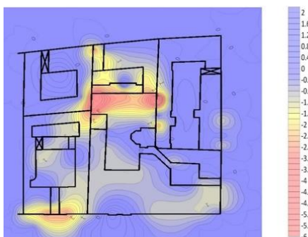
Figure 7. Diagram of deformations of the settlement of surrounding buildings.
