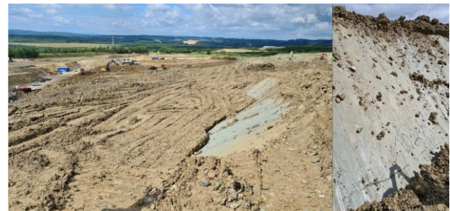
Figure 2. Main scarp upper edge of the landslide.
