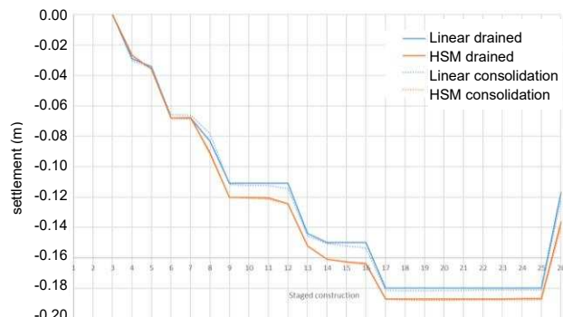
Figure 7. Comparison between linear and HSM calculation – settlement of HR centre.
