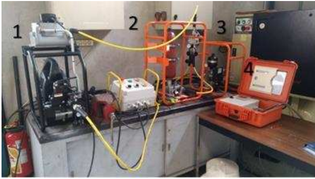
Figure 1. Connection of the device in running order: (1) hydraulic pump, (2) hydraulic accumulator, (3) controlled solenoid valve, (4), programmable automate (PLC).
