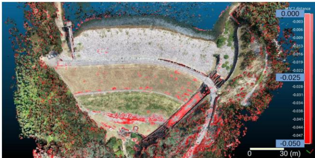
Figure 5. Settlements increments (2021-2022) in Lapa dam obtained by photogrammetric processing of high-resolution UAV images
