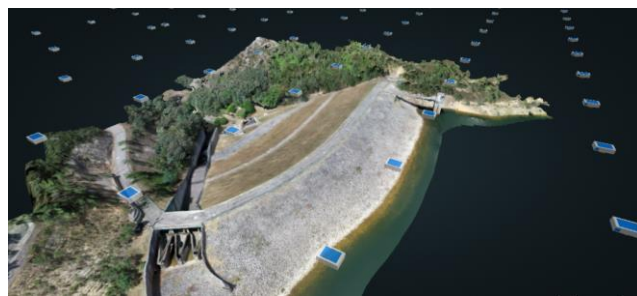
Figure 2. Textured model of Lapa dam and UAV positions, survey of 2022.
