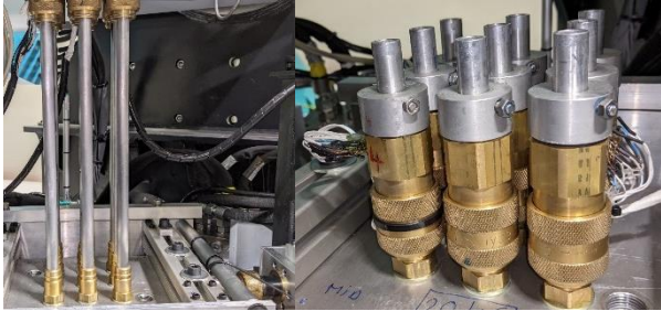
Figure 2. Plug-in method: open system before pile installation (left), coupled system after pile installation (right).
