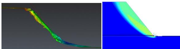
Figure 10. Slope deformation in physical (left) and numerical (right) models.
