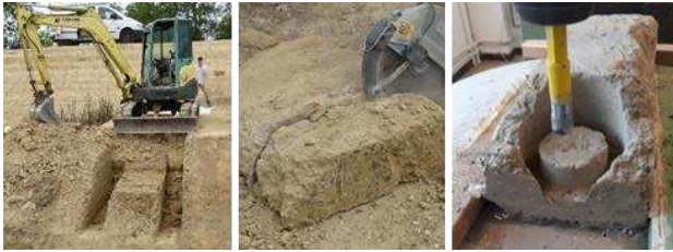
Figure 2. Left: View on the two trenches and the mechanical shovel. Middle: An extracted block re-sized using a floor saw for conditioning. Right: A re-sized block used to shape a sample by milling.
