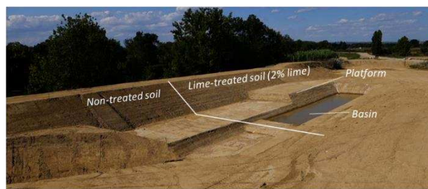
Figure 1. Aerial view of the Vidourle experimental levee. The platform and basin were also made with lime-treated soil and used for overflow test purposes.
