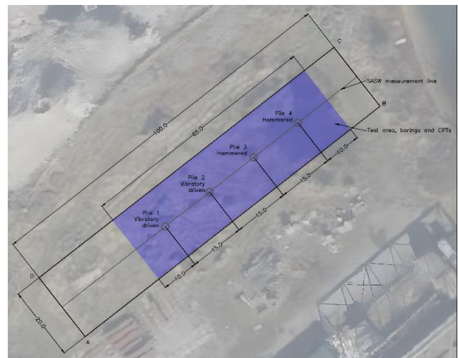
Figure 2. CPTs performed at the locations of the piles.
