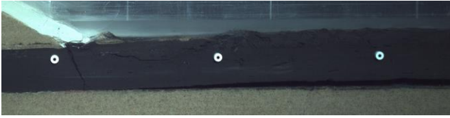
Figure 7. Uplift and separation of the cover layer.
