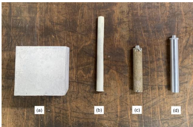
Figure 3. Samples used for roughness parameter comparison (a) concrete block (b) resin cast pile (c) sand coated pile (d) smooth aluminium pile.
