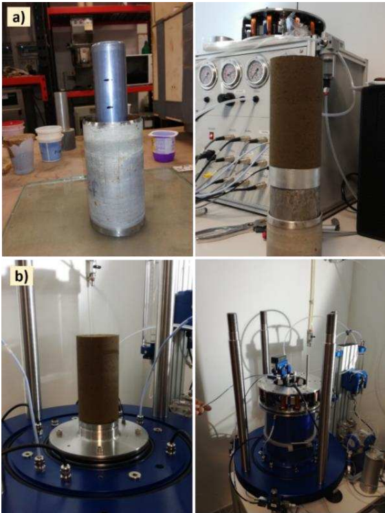
Figure 1. a) Soil specimen preparation; b) its assemblage within the RCTS equipment.
