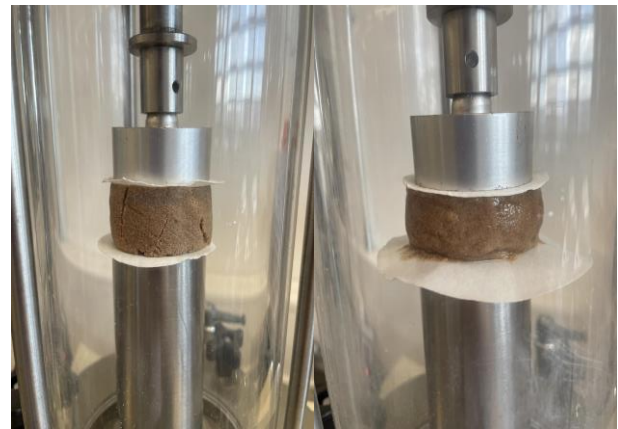
Figure 5. Failure mode of specimen after wetting (a) 1%CS; (b) 1%CS-MeOH-Ac2O.
