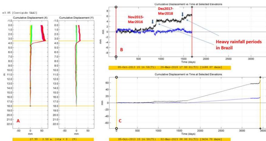
Figure 11. A) Cumulative displacements in the X (preferred direction of displacement) and Y axes of SAA1; B) Cumulative displacements in X (black) and Y (blue) axes over time at 3.5m depth, emphasizing acceleration during heavy rainfall; C) Cumulative displacements in X (black) and Y (blue) axes over time at 3.5m depth from 2013 to 2023.
