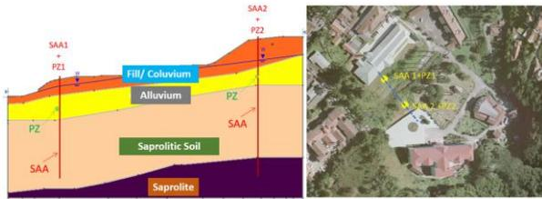
Figure 8. Cross-section with the location of the instruments (from top to bottom – Fill/Colluvium, Alluvium, Saprolitic soil, Sapolite).
