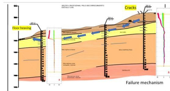
Figure 10. Illustration of the cumulative displacements in both ShapeArrays (left/right) according to the geological profile and installation site. Pathologies (cracks at the top and school floor heaving at the bottom). Location of vibrating wire piezometers and assumed position of the water table (NA) according to piezometric results. Understanding of the failure mechanism. (blue arrows).
