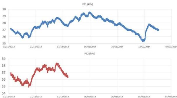
Figure 12. Pore pressure data recorded by vibrating wire piezometers (while operational).
