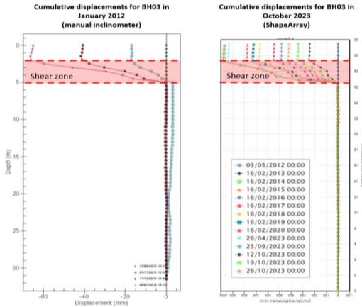
Figure 5. Comparison of cumulative displacement profiles between Jan/2012 and Oct/2023.
