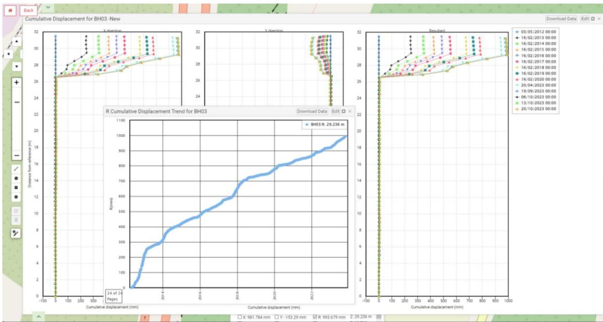
Figure 4. Cumulative displacement at BH03 in October 2023 and cumulative displacement trend.
