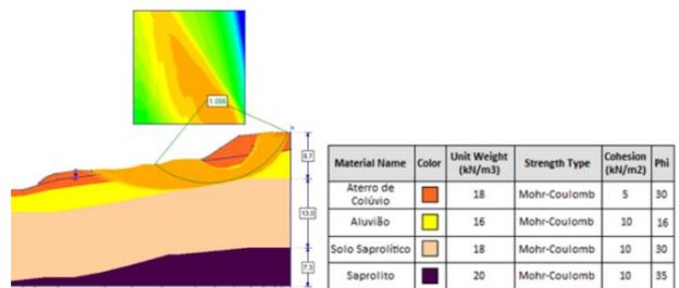
Figure 7. Results of the stability analysis (Morgenstern-Price Method - FS [1 to 1.5]). Material names translation from top to bottom: Fill/Colluvium, Alluvium, Saprolitic soil, Saprolite).
