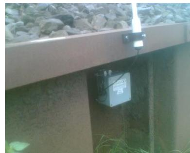
Figure 2. Wireless tiltmeter in a sheet pile wall.
