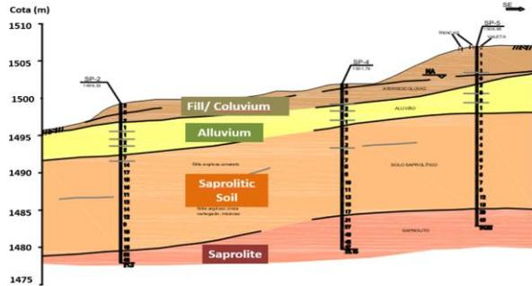
Figure 6. Geological profile of the study area (from top to bottom – Fill/Coluvium, Alluvium, Saprolitic soil, Saprolite).
