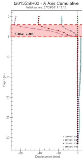
Figure 1. Manual inclinometer results for BH03 Jan/2012.
