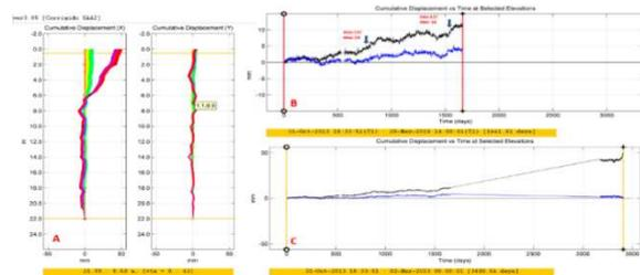
Figure 9. A) Cumulative displacements in the X (preferred direction of displacement) and Y axes of SAA2; B) Cumulative displacements in X (black) and Y (blue) axes over time at 1.0m depth, emphasizing acceleration during heavy rainfall; C) Cumulative displacements in X (black) and Y (blue) axes over time at 1.0m depth from 2013 to 2023.
