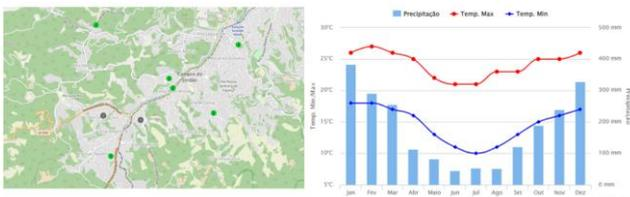
Figure 13. Left- Rain Gauge location (Green circles); Right - the average behaviour of rainfall (blue histogram) and temperature (min-blue line/max- red line) throughout the year at Campos de Jordão city— Source: CEMADEN.
