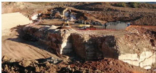
Figure 3. View of abrupt transitions between landfill zones and vertical faces of the limestone quarry.
