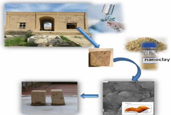
Figure 2. Nano-Spray for Historic Buildings and Earth Houses (Khaksar et al., 2023).
