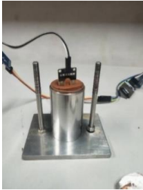
Figure 2. Calibration process of soil water content sensor.
