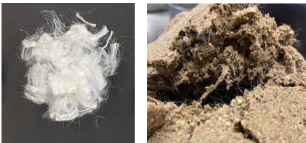
Figure 1. The polypropylene fibres with 18 mm longest and soil mixed with 0.3% of the fibres.
