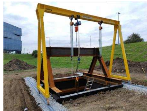
Figure 2. Testing container, loading frame and auxiliary crane.
