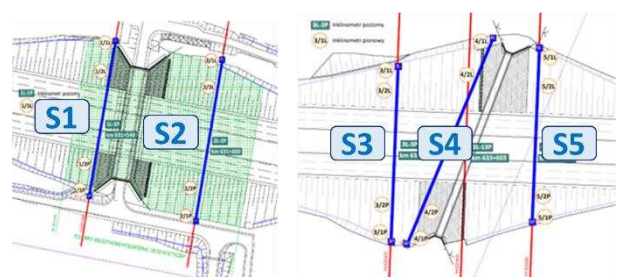
Figure 11. Selected locations of measurement cross-sections (S1 – S5) within the embankment - top view.
