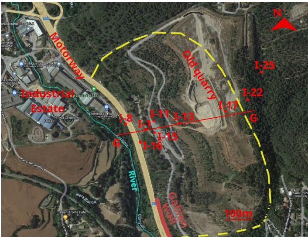
Figure 1. Layout of the motorway and the old quarry on the upper part of the slope (right-hand side). The picture also shows the industrial estate on the opposite side of the road with respect to the unstable slope (discontinuous line) and the location of Section G object of this study (Google maps image).
