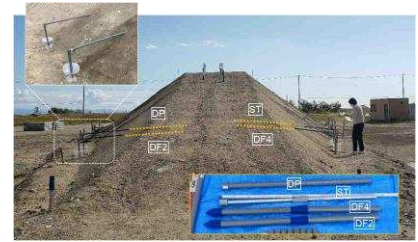
Figure 5. Alignment of drainage pipe.
