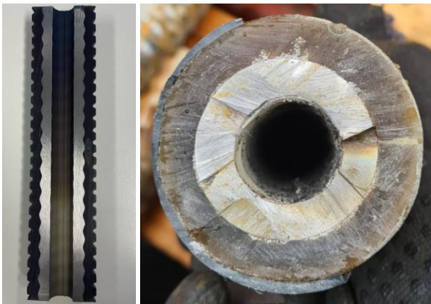
Figure 3. Developed double-corrosion-protection self-drilling tension element (DCP-SBZ), top: schematic, bottom: longitudinal and sectional cross section.
