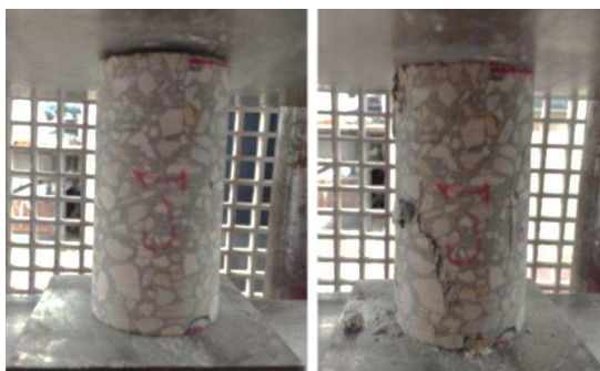
Figure 6. Uniaxial compression-strength testing – UCS.
