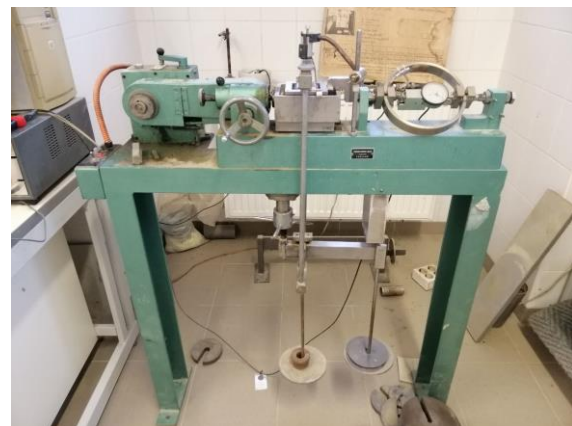
Figure 3. Direct shear test (The Laboratory of Geotechnics and Engineering Geology at BME University, Hungary).
