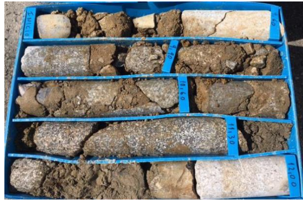
Figure 3. Soil samples taken from Geotechnical Layer 2. Granite boulders wrapped in sandy clay matrix.
