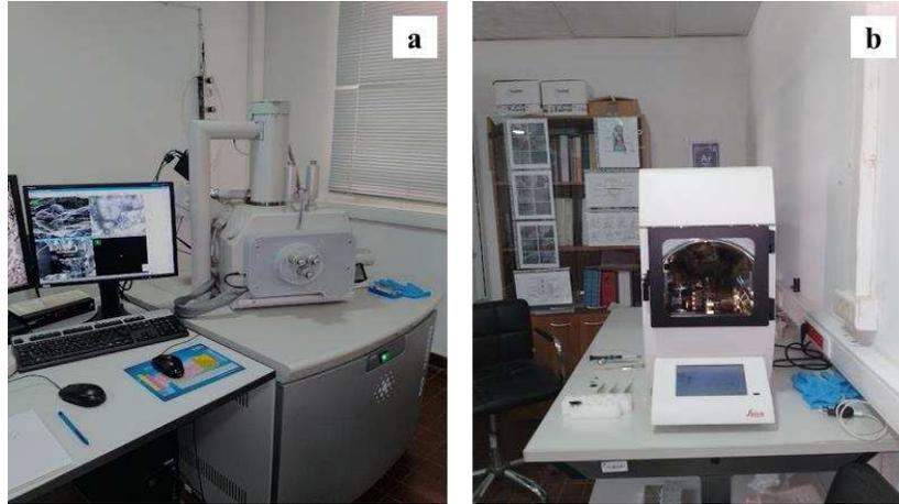
Figure 3. Instrumentation for Microscopic Analysis: (a) electronic scanning microscope QUANTA 650; (b) metallizer ACE 200.
