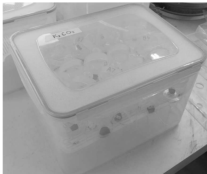
Figure 2. Airtight container with saturated K 2 CO 3 solution
