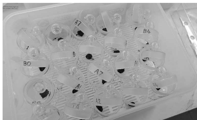
Figure 3. Batch of soil samples equalising to K 2 CO 3 solution
