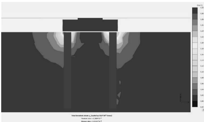
Figure 8. Shear strain output for horizontal loading (all piles and pile cap).
