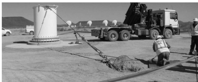
Figure 3. Prototype pull test setup
