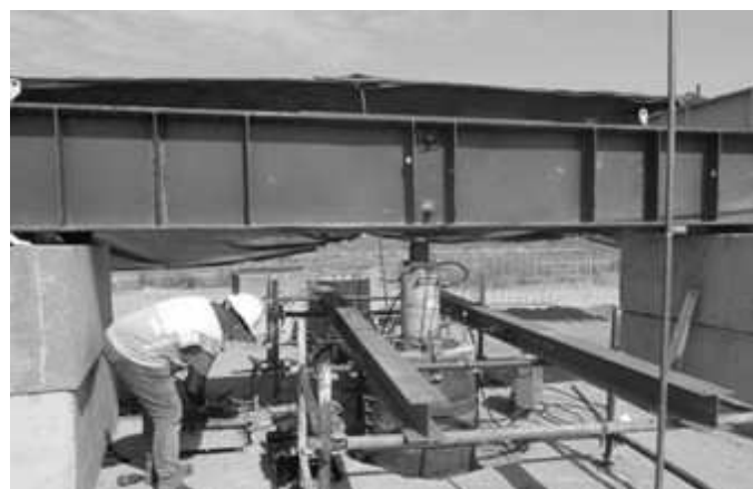
Figure 4. Pile load test setup, 2024
