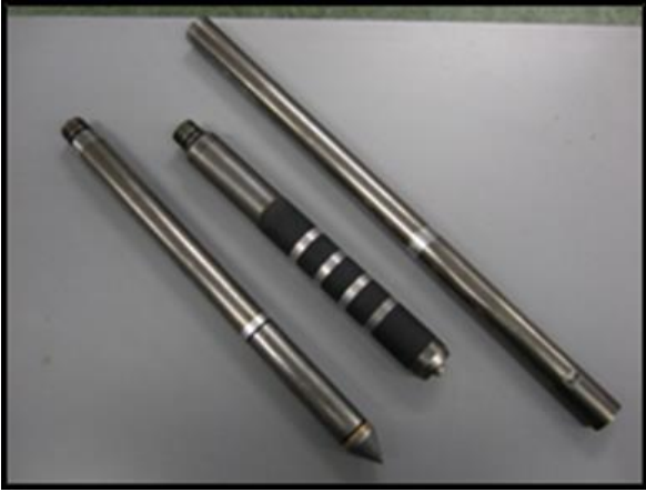
Figure 2 Example of R-CPTU probe (NIFS-report 2015-126).
