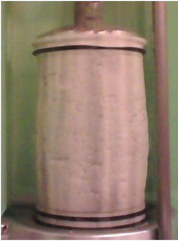
Figure 7 Specimen shape at failure ( \varepsilon_l = 10\% ) for B34 (C), Type 3, H/D=2 , D = 70\text{mm} .
