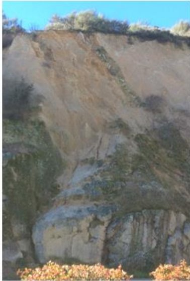
Figure 2 Example of granitic residual soil slopes in the Covilhã region with the parent rock at the bottom.
